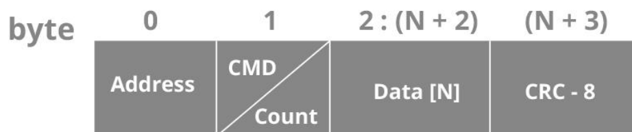
Figure 12. Frame structure for Evo 64px commands
